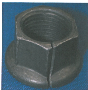
Figure 1 – Example of longitudinal crack reproduced from Reference (1)
