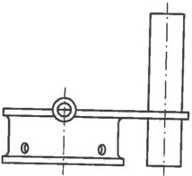
FIG 1 - SAB NOSEWHEEL STEERING ADAPTOR (SAB PT. NO. 918-607)
