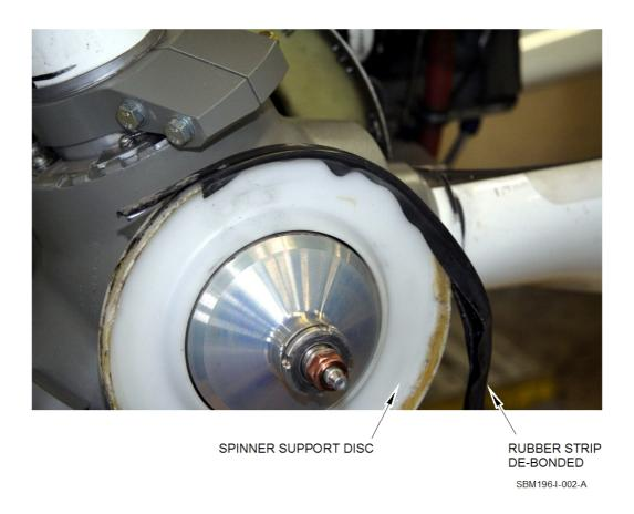
Figure 2 De-bonded rubber strip (T67M200)
