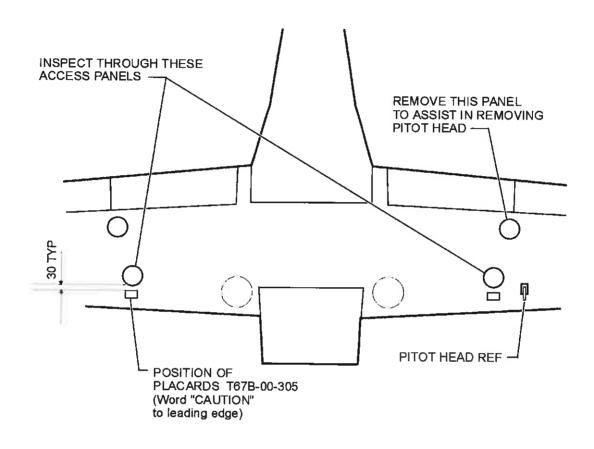
Figure 2 Showing Access Panels and Placard Position
