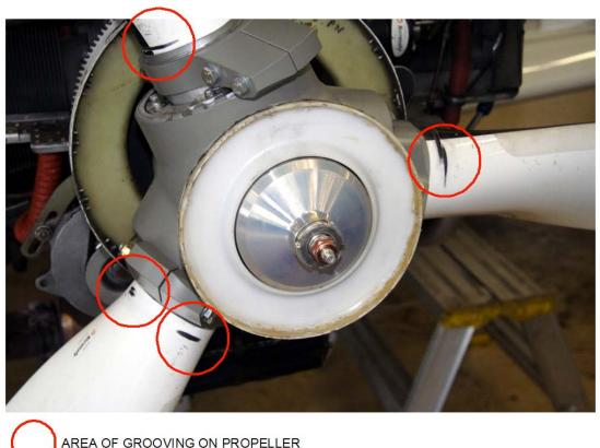
AREA OF GROOVING ON PROPELLER
