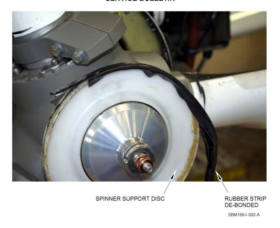
Figure 2 De-bonded rubber strip (T67M200)
