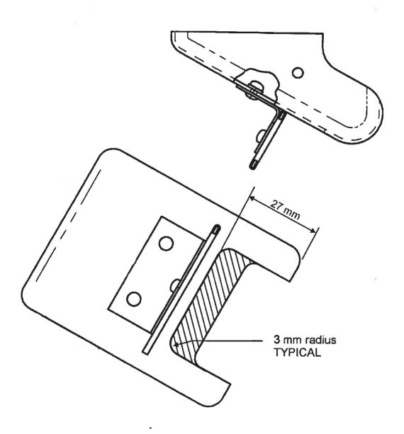
FIGURE 2 LATCH BLOCK COVER ON FIXED CANOPY
