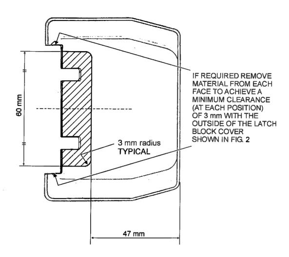
FIGURE 3 LATCH COVER ON THE MOVEABLE CANOPY
