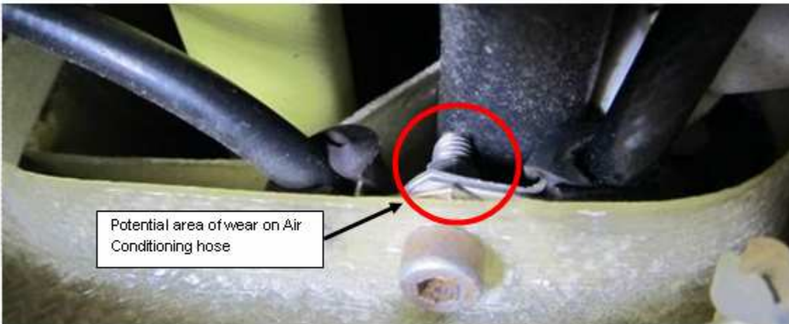
Figure 2 Plan view of air conditioning installation aft of Frame 5
