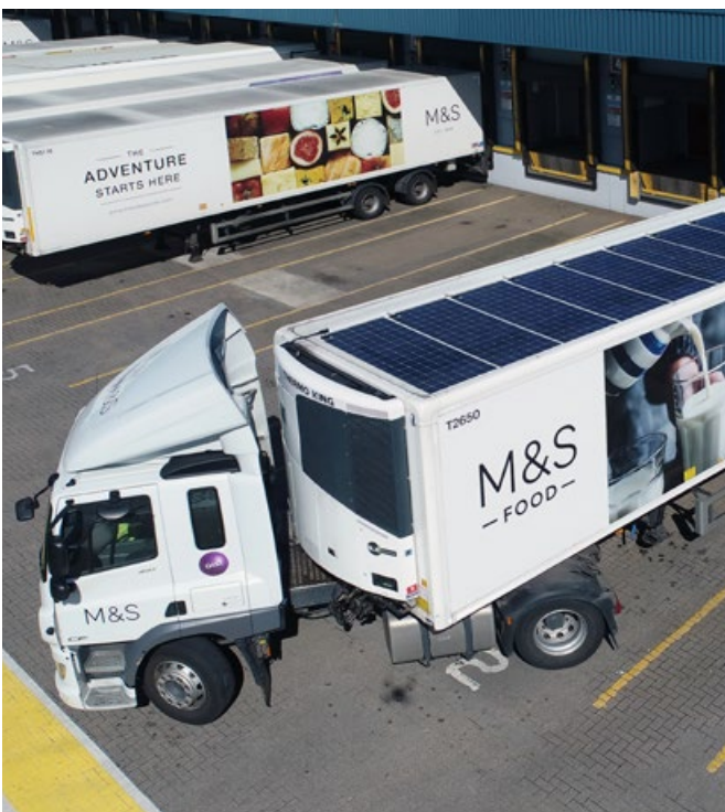
Thermo King Fridge Unit on an M&S Trailer
